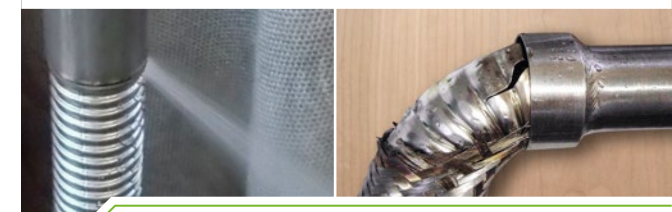
Leakage after pressure impulse test, damage after burst test (l. to r.)
