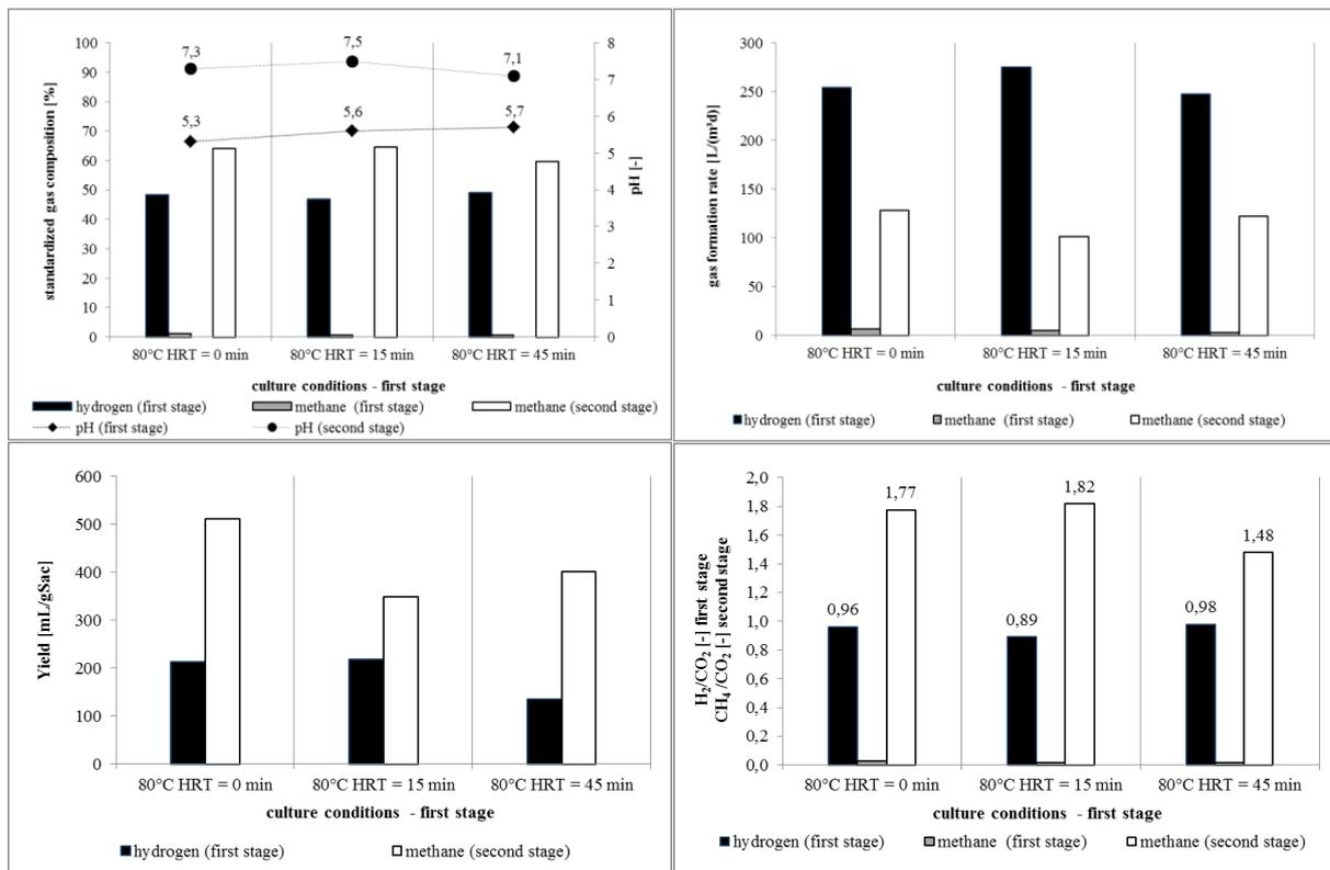
Figure 5. Comparison between standardizes gas composition (top left), gas formation rate of CH<sub>4</sub> and H<sub>2</sub> (top right), the Yield of CH<sub>4</sub> and H<sub>2</sub> (bottom left) and the ratio of CH<sub>4</sub> to CO<sub>2</sub> or H<sub>2</sub> to CO<sub>2</sub> (bottom right) of first and second stage depending on the duration of thermal digestate denaturation
