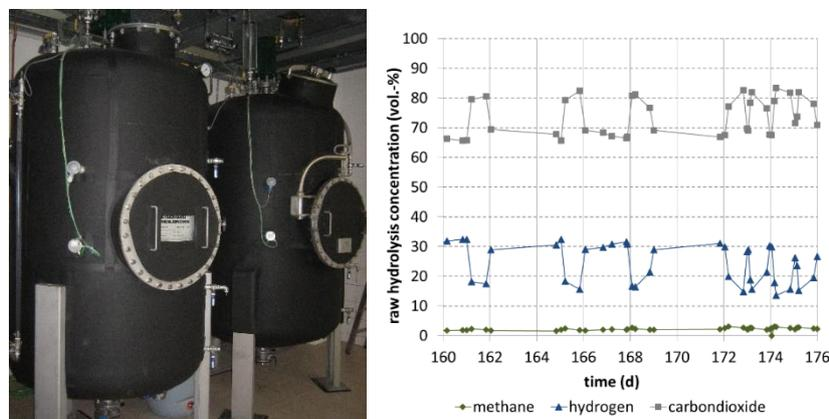
Figure 2. Experimental setup of already established cyclic two-stage biogas plant for synthesis of bio-hydrogen and bio-methane (left) with steady state raw gas concentrations (right)
