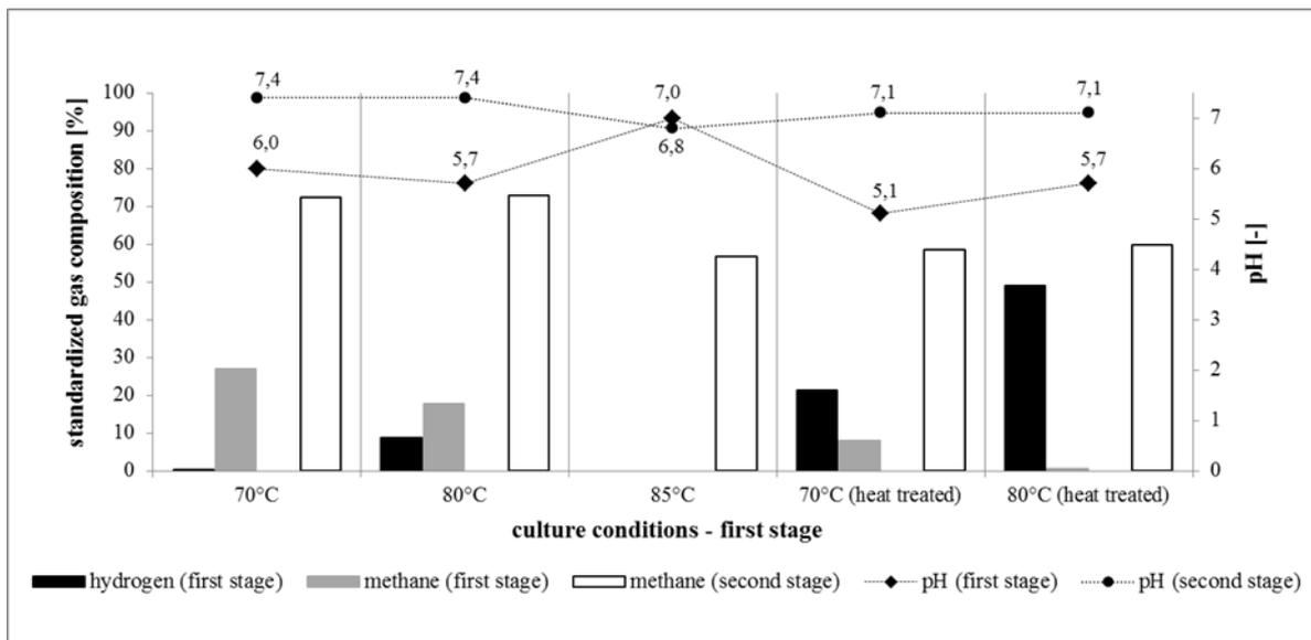
Figure 4. Comparison between gas composition and pH value of first and second stage in relation to varying culture temperatures of the first stage and with/without heat treatment of the digestate; first stage: hydrogen fermentation; second stage: methane fermentation
