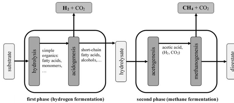
Figure 1. Simplified scheme of bio-hydrogen and bio-methane production
