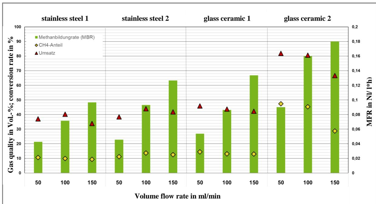
Figure 7: Conversion rate, proportion of methane and methane formation rate according to Gas injection system and volume flow rate
