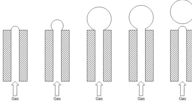
Figure 2: Genesis of bubbles at an injector [10]
