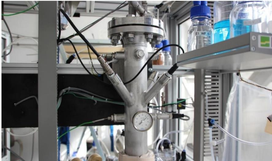
Figure 5: section of the pressurized bubble column
