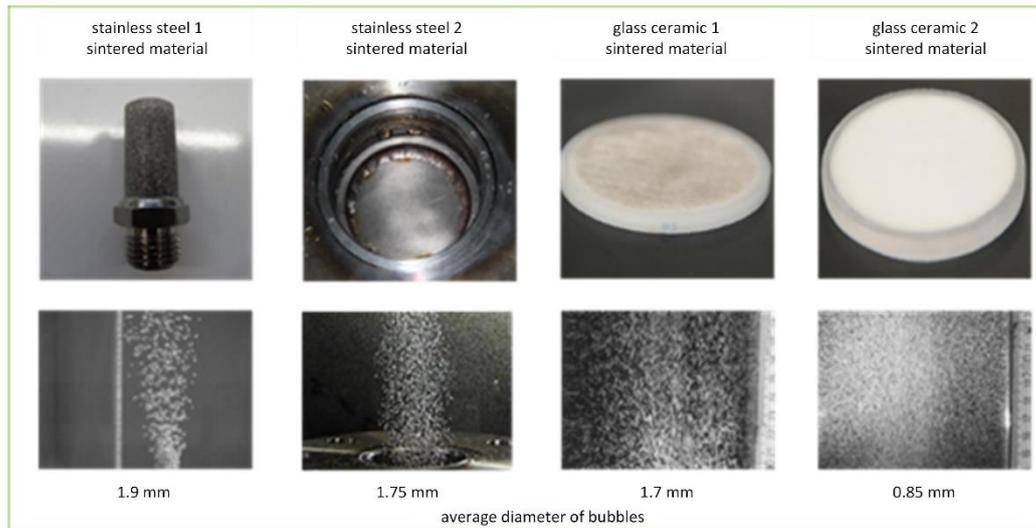
Figure 6: bubble images and average diameter for different gas injectors
