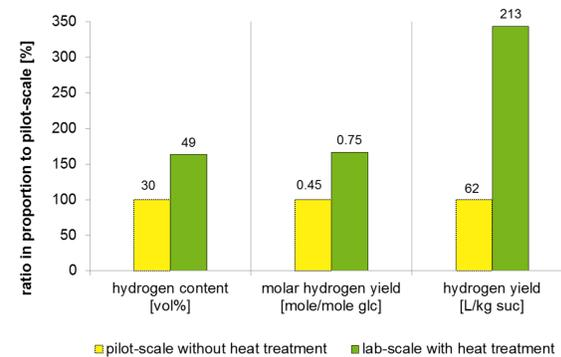
Figure 6. Optimization due to thermal treatment in lab-scale experiments compared to pilot scale (bar labels show absolute values)
