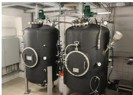
Figure 2. Pilot biogas plant - 2 m<sup>3</sup> scale
