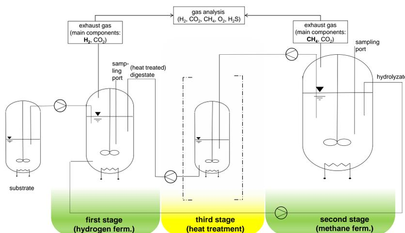
Figure 4. Experimental setup for optimization of the established process-setup
