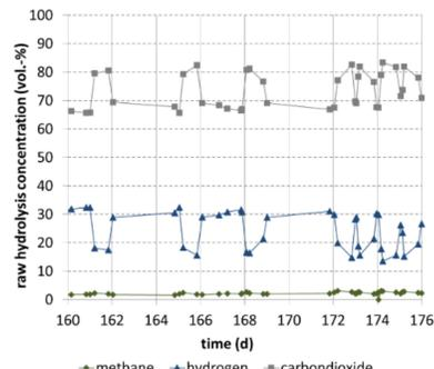
Figure 3. Raw-gas concentration (hydrolysis)
