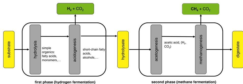
Figure 1. Simplified scheme of biohydrogen and biomethan (biogas) production
